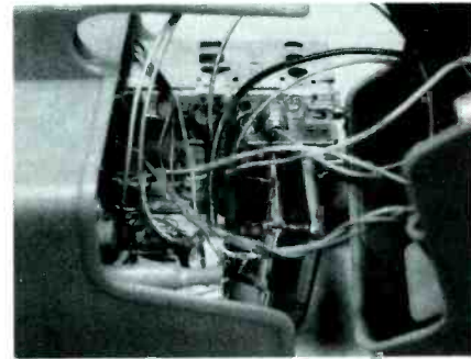
Fig. 5 There is no excess space inside the Master Subber. Most of the components not in the tuner are inside two small modules.
